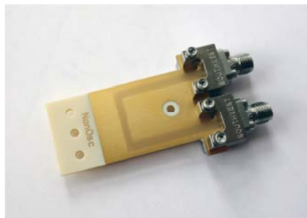
Coplanar Waveguide (CPW) for room temperature PhaseFMR
